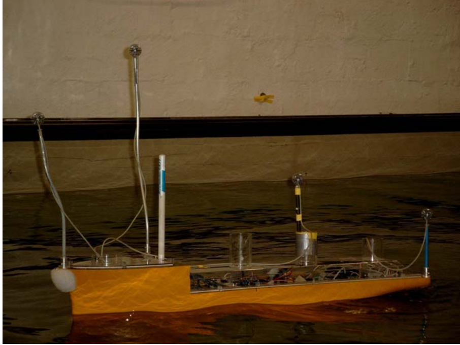
Figure 2: Cybership II, a model supply ship, Froude scaled 1:70.
