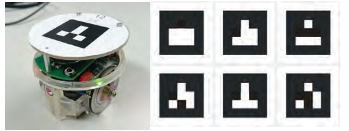
Fig. 10. E-puck mobile robot (left) and markers used for identification (right).
