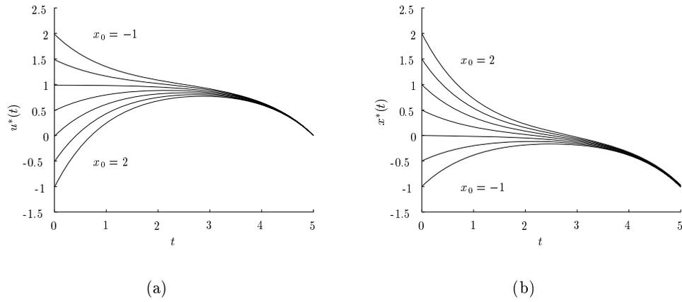
Figure D.1: Influence of initial state  $x_0$  with free control ( $u$ ): (a) optimal control path  $u^*(t)$  and (b) optimal state path  $x^*(t)$  for a range of initial states  $x_0$  from -1 to 2 with stepsize  $\frac{1}{2}$ .
