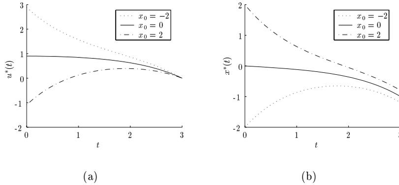
Figure A.1: Numerical example of the free system behavior ( $u$ ): (a) the optimal open loop control law  $u^*(t)$  and (b) the optimal state function  $x^*(t)$  for several values of the initial state  $x_0$ .
