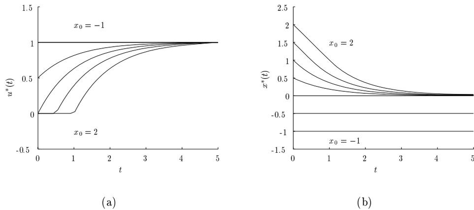
Figure D.4: Influence of initial state  $x_0$  with limited control ( $u - d$ ): (a) optimal control path  $u^*(t)$  and (b) optimal state path  $x^*(t)$  for a range of initial states  $x_0$  from -1 to 2 with stepsize  $\frac{1}{2}$ .
