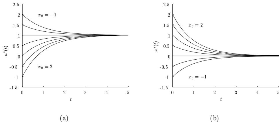
Figure 5.4: Numerical example of: (a) the optimal open loop control path  $u^*(t)$  and (b) the optimal state path  $x^*(t)$  for the free system ( $u - d$ ) for a range of initial states  $x_0$  from -1 to 2 with step size  $\frac{1}{2}$ .
