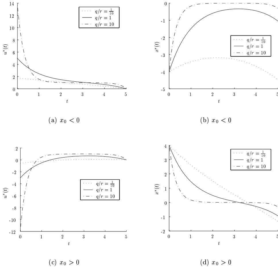
Figure D.6: Influence of cost parameters  $q$  and  $r$  with free control ( $u$ ) on the optimal control path  $u^*(t)$  and the optimal state path  $x^*(t)$ .
