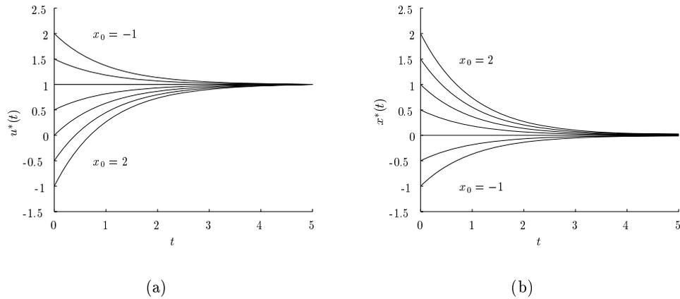
Figure D.2: Influence of initial state  $x_0$  with free control ( $u - d$ ): (a) optimal control path  $u^*(t)$  and (b) optimal state path  $x^*(t)$  for a range of initial states  $x_0$  from -1 to 2 with stepsize  $\frac{1}{2}$ .
