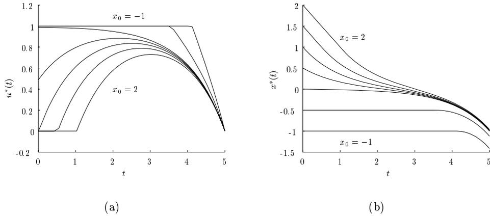
Figure 5.5: Numerical example of: (a) the optimal open loop control path  $u^*(t)$  and (b) the optimal state path  $x^*(t)$  for the limited system ( $u$ ) for a range of initial states  $x_0$  from -1 to 2 with step size  $\frac{1}{2}$ .
