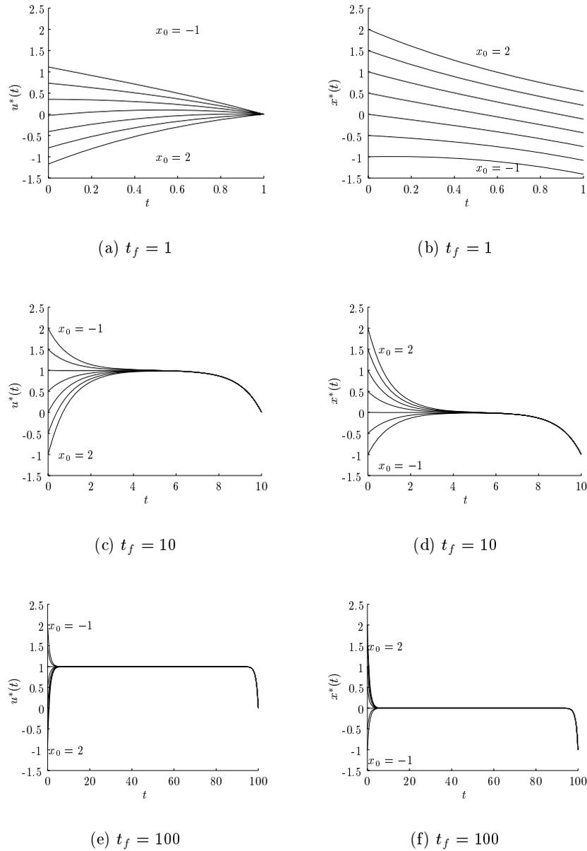
Figure D.5: Influence of final time  $t_f$  with free control ( $u$ ) on the optimal control path  $u^*(t)$  and the optimal state path  $x^*(t)$  for a range of initial states  $x_0$  from -1 to 2 with stepsize  $\frac{1}{2}$ .
