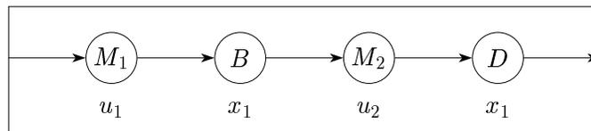
Figure 4.1: A two-machine flow shop  $WW$ .
