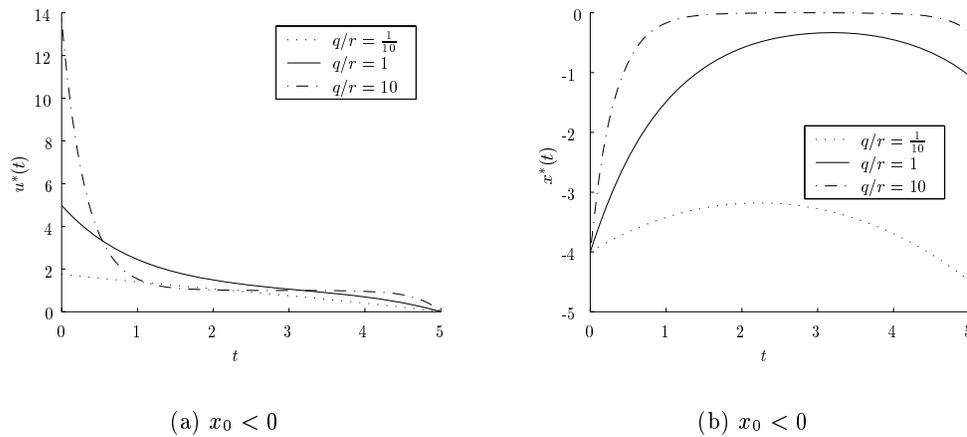
Figure 5.7: Influence of cost parameters  $q$  and  $r$  with free control ( $u$ ) on (a) the optimal control path  $u^*(t)$  and (b) the optimal state path  $x^*(t)$ .
