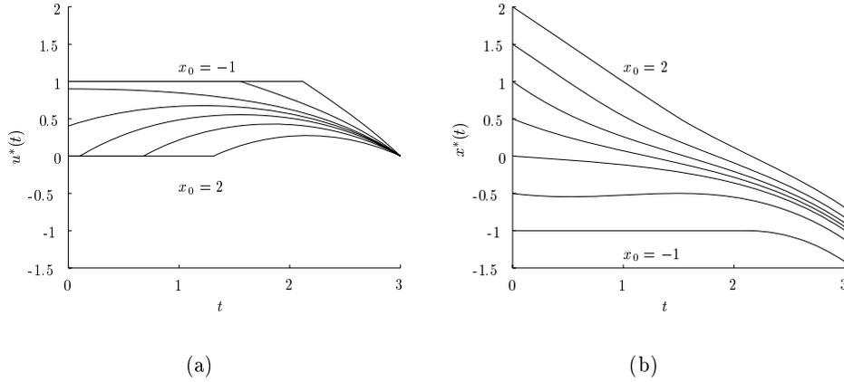
Figure B.3: Numerical example of: (a) the optimal open loop control law  $u^*(t)$  and (b) the optimal state function  $x^*(t)$  for the limited system for a range of initial states  $x_0$  from -1 to 2 with step size  $\frac{1}{2}$ .
