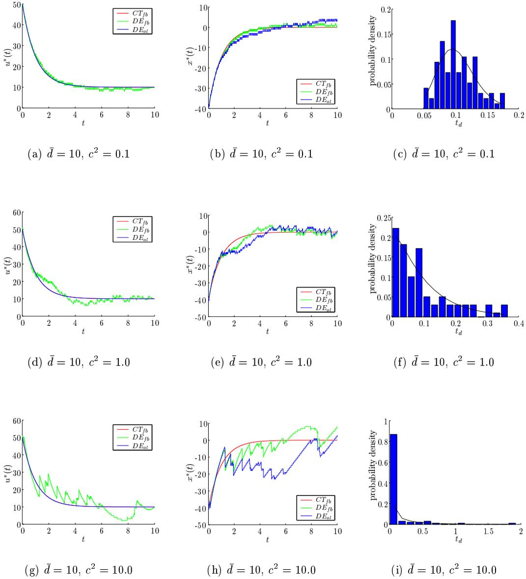
Figure D.18: Open loop and feedback control in the stochastic case with free control ( $u - d$ ) and negative initial state  $x_0$ . Control and state paths are shown for several values of inter request time variability: (a, b, c) lowly variable, (d, e, f) moderately variable, and (g, h, i) highly variable. Validity of the flow model is critical with an average demand rate  $\bar{d} = 10$ .
