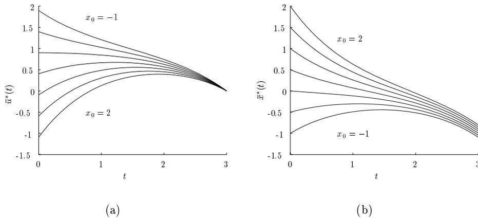
Figure B.1: Numerical example of: (a) the optimal open loop control law  $\bar{u}^*(t)$  and (b) the optimal state function  $\bar{x}^*(t)$  for the free system for a range of initial states  $x_0$  from -1 to 2 with step size  $\frac{1}{2}$ .
