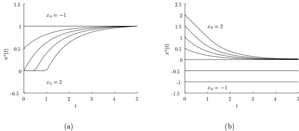
Figure 5.6: Numerical example of: (a) the optimal open loop control path  $u^*(t)$  and (b) the optimal state path  $x^*(t)$  for the limited system  $(u - d)$  for a range of initial states  $x_0$  from -1 to 2 with step size  $\frac{1}{2}$ .
