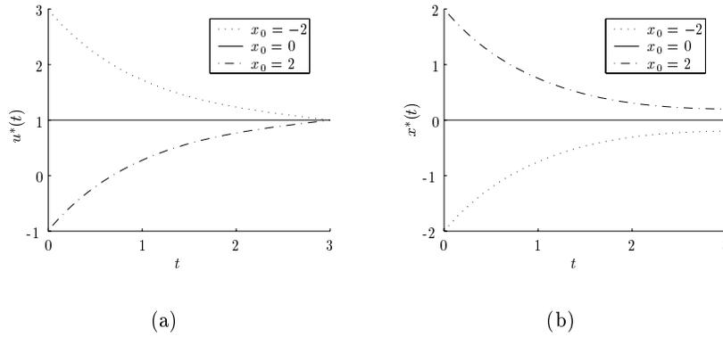
Figure A.2: Numerical example of the free system behavior ( $u - d$ ): (a) the optimal open loop control law  $u^*(t)$  and (b) the optimal state function  $x^*(t)$  for several values of the initial state  $x_0$ .
