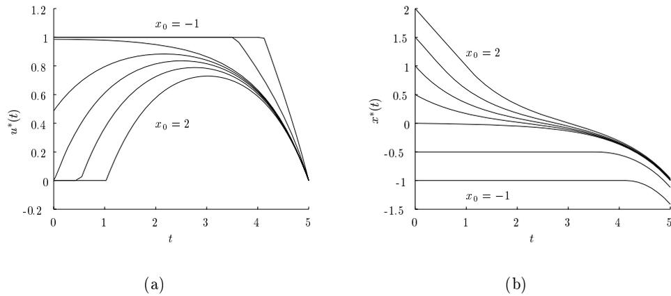
Figure D.3: Influence of initial state  $x_0$  with limited control ( $u$ ): (a) optimal control path  $u^*(t)$  and (b) optimal state path  $x^*(t)$  for a range of initial states  $x_0$  from -1 to 2 with stepsize  $\frac{1}{2}$ .
