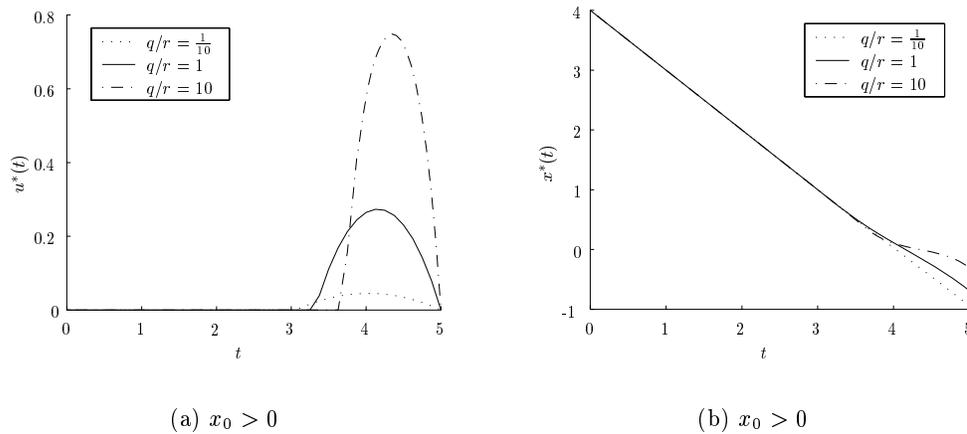
Figure 5.8: Influence of cost parameters  $q$  and  $r$  with limited control ( $u$ ) on (a) the optimal control path  $u^*(t)$  and (b) the optimal state path  $x^*(t)$ .
