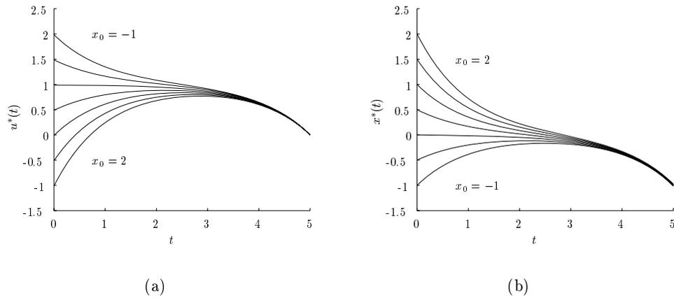
Figure 5.3: Numerical example of: (a) the optimal open loop control path  $u^*(t)$  and (b) the optimal state path  $x^*(t)$  for the free system ( $u$ ) for a range of initial states  $x_0$  from -1 to 2 with step size  $\frac{1}{2}$ .
