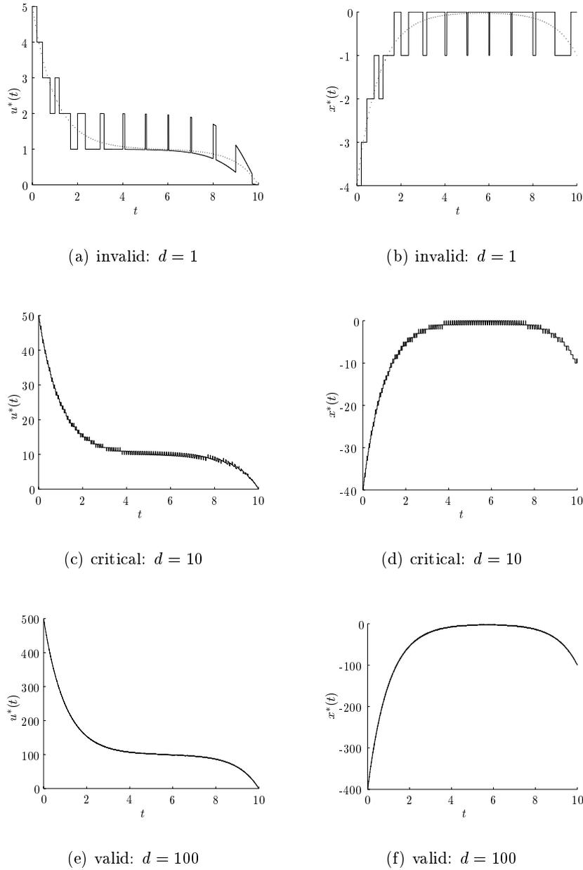
Figure 5.9: Optimal control paths  $u^*(t)$  and optimal state paths  $x^*(t)$  with free control ( $u$ ) for demand rates  $d$  where the flow model is (a, b) invalid, (c, d) critical, and (e, f) valid and with negative initial states  $x_0$ .
