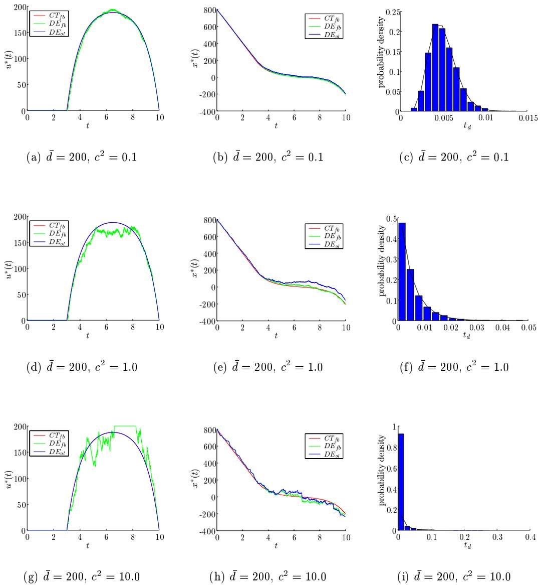
Figure D.19: Open loop and feedback control in the stochastic case with limited control ( $u$ ) and positive initial state  $x_0$ . Control and state paths are shown for several values of inter request time variability: (a, b, c) lowly variable, (d, e, f) moderately variable, and (g, h, i) highly variable. Validity of the flow model is critical with an average demand rate  $\bar{d} = 200$ .
