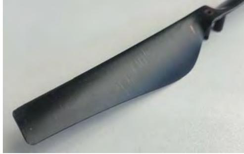
**Figure 3.2:** The rotor blade of the AR Drone 2.0
