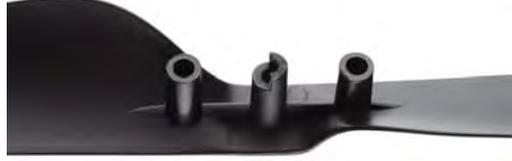
**Figure 5.8:** Detailed view of the rotor blade at the hub. In the middle of the blade the rib which gives stiffness to the rotor hub. The rib extends into the blades and might act as a fictional hinge.
