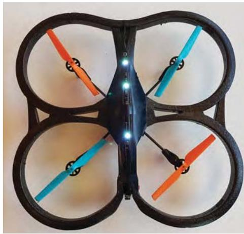
**Figure 6.6:** Parrot AR Drone 2.0 with protective hull and LED identifiers.
